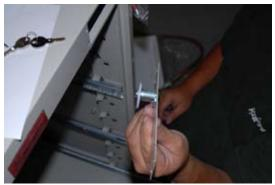
10. Pull key out and put plate with lock in place in the cart's frame
