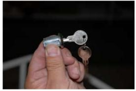
4. Hold lock so key is upright with teeth of key pointing upwards. (Key must turn to right and stop)
