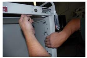
11. Raise lock bar up so plastic cam meets up with horizontal extension of lock bar.
