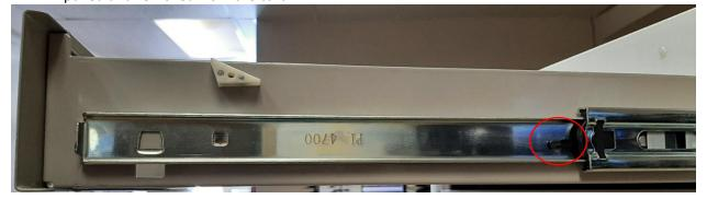
3 Grasp the extended portion of the slide attached to the cart and twist the slide towards the center of the cart then pull up on the slide to free it from the cabinet.
