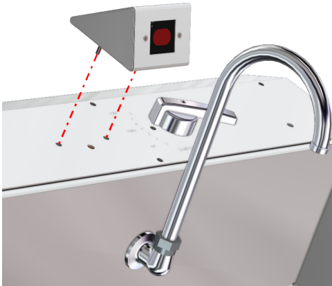
Fig. 14: Attach IR sensor housing to header
