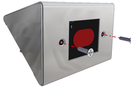
Fig. 11: Secure IR sensor to housing
