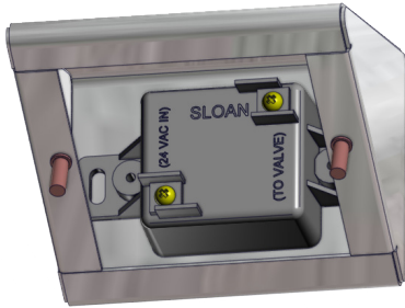
Fig. 10: Place IR sensor in housing
