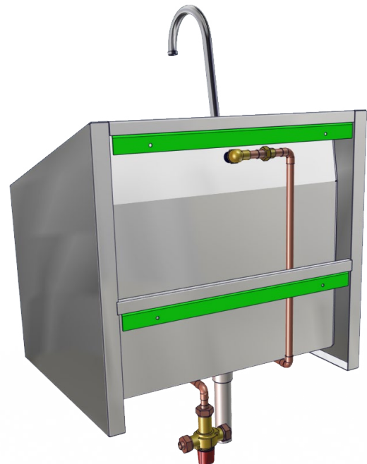
Fig. 6: Z Brackets on Sink
